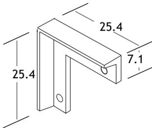
**Steel Miter Bracket for Reflector Shells**
