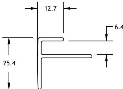
**Extrusion Profile for Assembly #790004**
