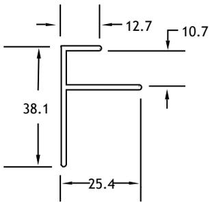
**Extrusion Profile for Assembly #790003**
